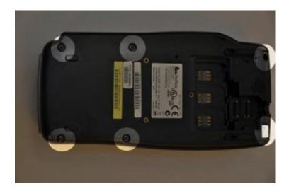
There are six screw positions on the back facia. Four are visible below the general information label. Two more are located under the back panel, one is covered by the VeriFone security seal.
