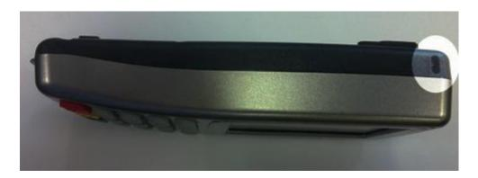
A Secure Tether Adapter is located on the left facia of the device to allow secure tether options to be attached to the device.
